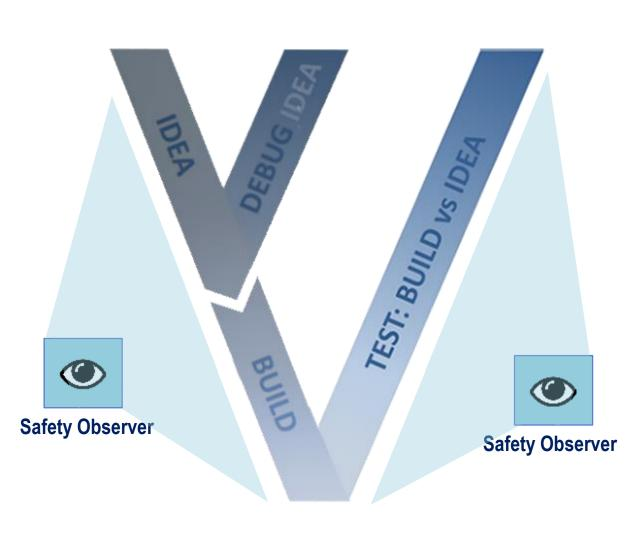
Then, during all the development process the safety properties can be reused as "Virtual Guides" (Observers) that will detect automatically violations of the Safety
